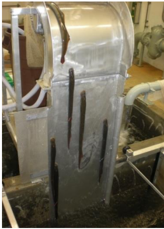
Figure 35. Photos of experimental wetted wall collector show lamprey ascending during a trial.
