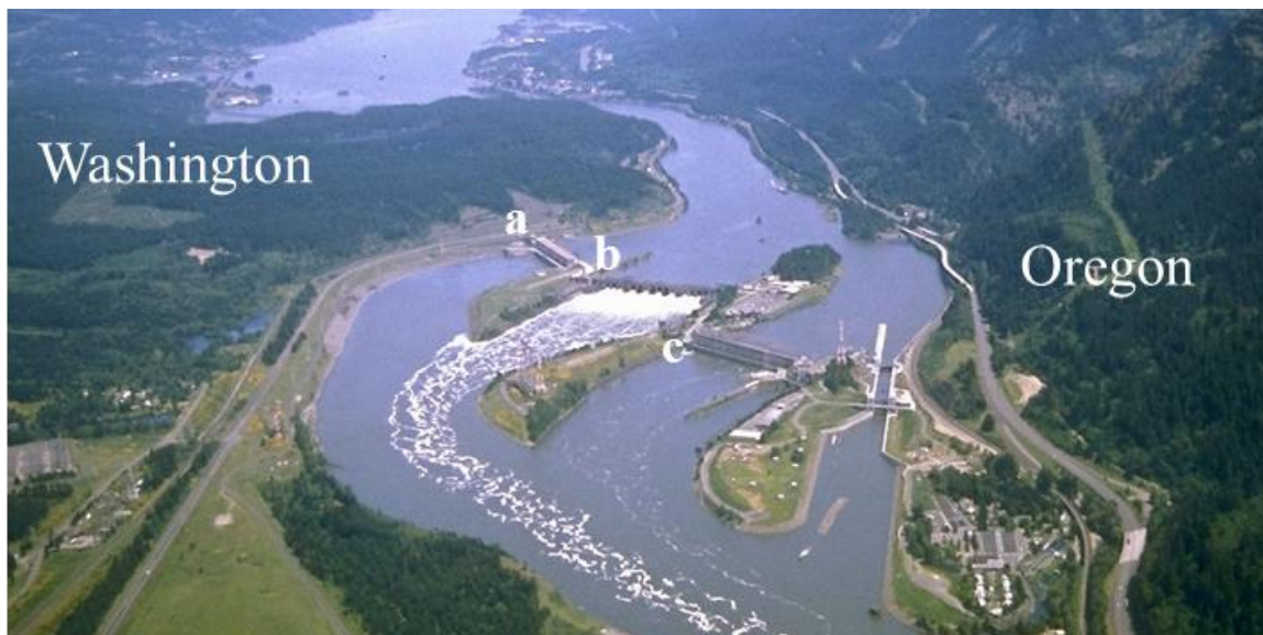
Figure 1. Aerial photo showing configuration of Bonneville Dam with approximate location of fishways at: (a) Washington Shore, (b) Cascades Island, and (c) Bradford Island.
