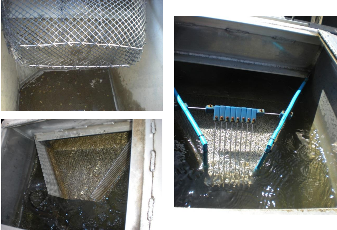
Figure C4. Examples of different fyke entry designs for rest boxes in the Cascades Island LPS.
